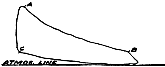
FIG. 121.—Gas Engine Indicator Card. This diagram is an average good card, showing, however, some slight fluctuations in the lines. The explosion line is from C to A; the expansion, from A to B; the exhaust at B. The suction stroke generally approximates the atmospheric line, from which the curve of compression rises to C.
